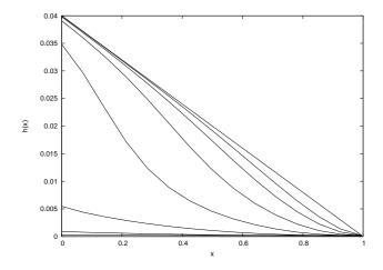
Figure 1: Evolution along time of a perturbation of the rolling layer at the bottom of the slope. The different lines indicate the profile of the static layer at successive instants of time. In this case, it can be seen that the thickness of the static layer decreases until it is almost zero. The parameters of the model were v = 0.1, D = 0.1 and  $\gamma = 0.01$
