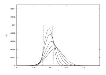
Figure 3: Evolution along time of a perturbation of the rolling layer in the middle of the slope. Again, the dashed line indicates the initial profile of the rolling layer, while the different continuous lines indicate its successive distributions. The region affected by the avalanche includes part of the cells above the initial perturbation. The parameters of the model were the same as in Figure 2.
