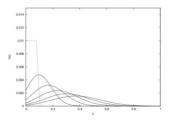
Figure 2: Evolution along time of a perturbation of the rolling layer on top of the slope. The dashed line indicates the initial profile of the rolling layer, while the different continuous lines indicate its successive distributions. The static layer has a slope to the right, slightly lower than the *repose angle*. The parameters of the model were v = 2.5, D = 0.1 and  $\gamma = 0.01$ .
