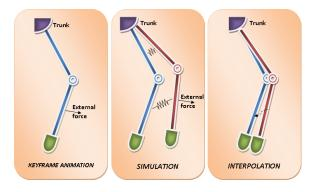
Figure 2: Scheme of an animation of the arm. When a force acts on an extremity, a physic model (bones in red) is activated and linked to the key-frame animation (bones in blue) using springs. When the force ceases, and the physics model is close to the key-frame animation, then it is interpolated.
